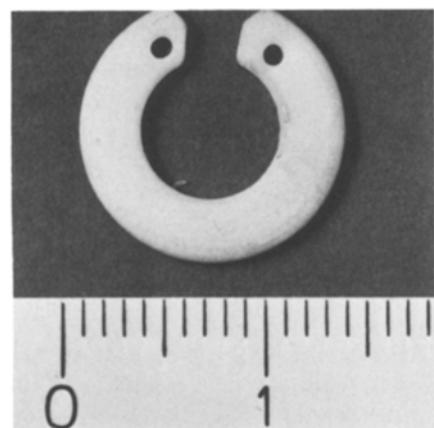
Fig. 1. The Teflon horse shoe ring used for obstruction (inner diameter 6 mm)
